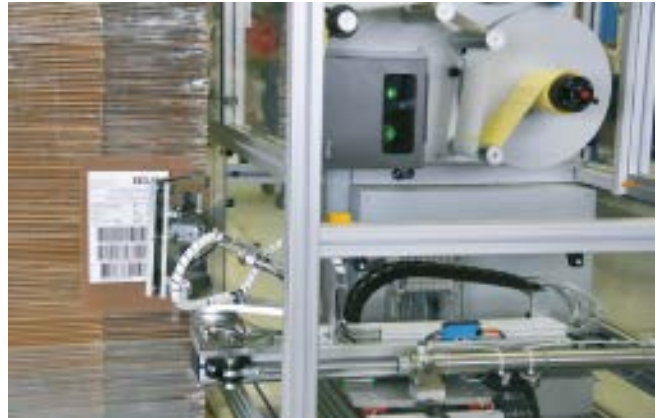
Pallet labeling (one stop for two sides)
