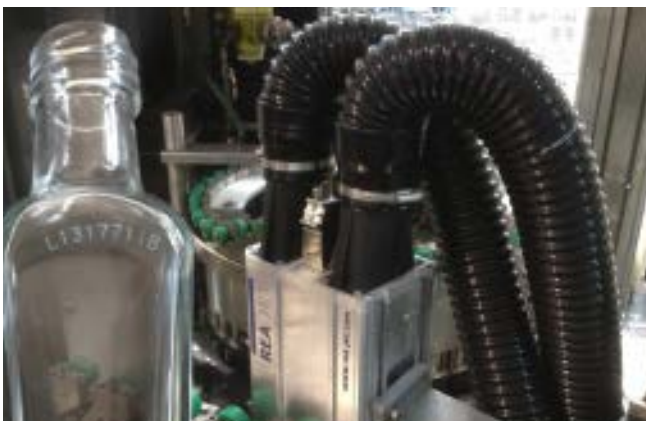
Coding and marking of glass with CO 2 laser IP65
