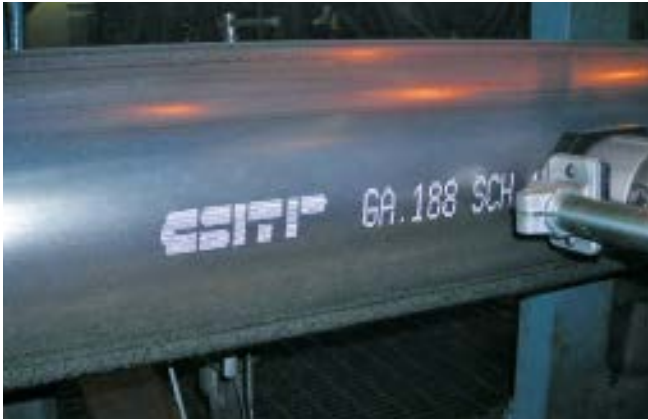
Coding and marking of pipes (steel, plastic etc.)
