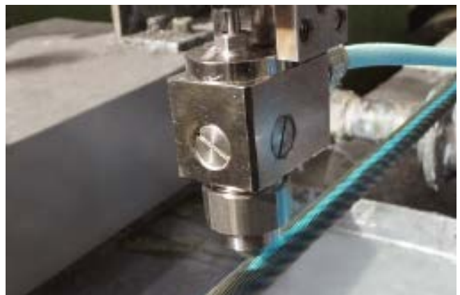
Color marking of wire cables
