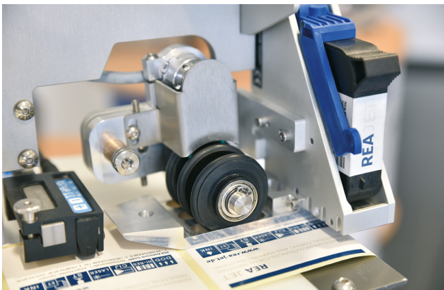
REA LABEL ES with integrated REA JET HR
