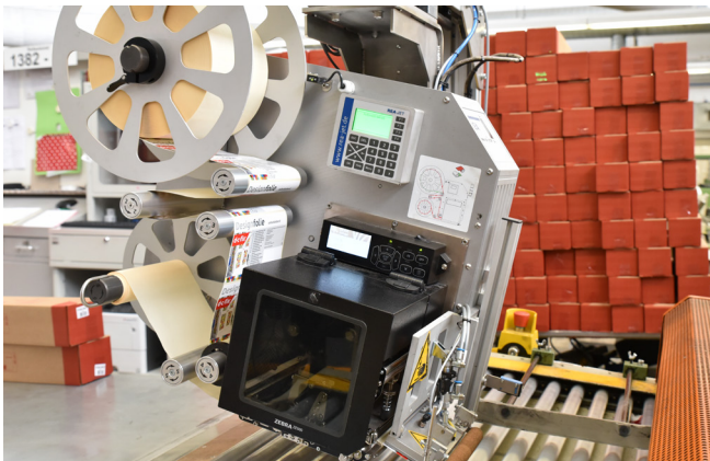
Print and apply system for wrap-around labeling
