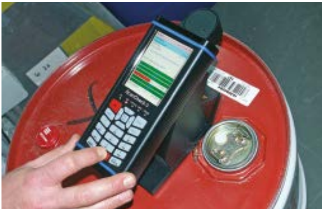
Verification of barcodes on metal drums
