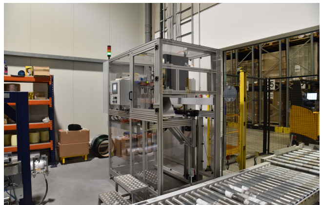
A4 Pallet Labeler Unit with vertical movement
