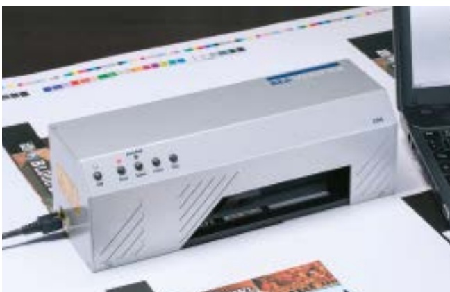
Measuring of barcodes on print sample sheets
